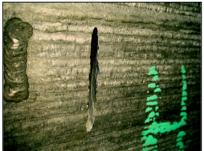
Figure 2. Close-up of a grind method cut. A previously re-welded cut is seen on the left.
