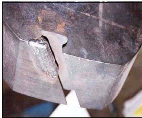
Figure 4. Mockup weld for repair of combustion turbine compressor disc.
