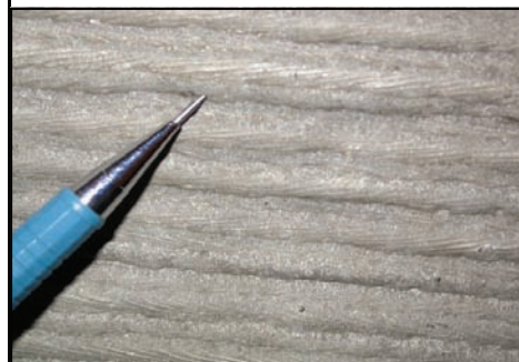
Type 312 Stainless Steel GMAW Light General Corrosion
