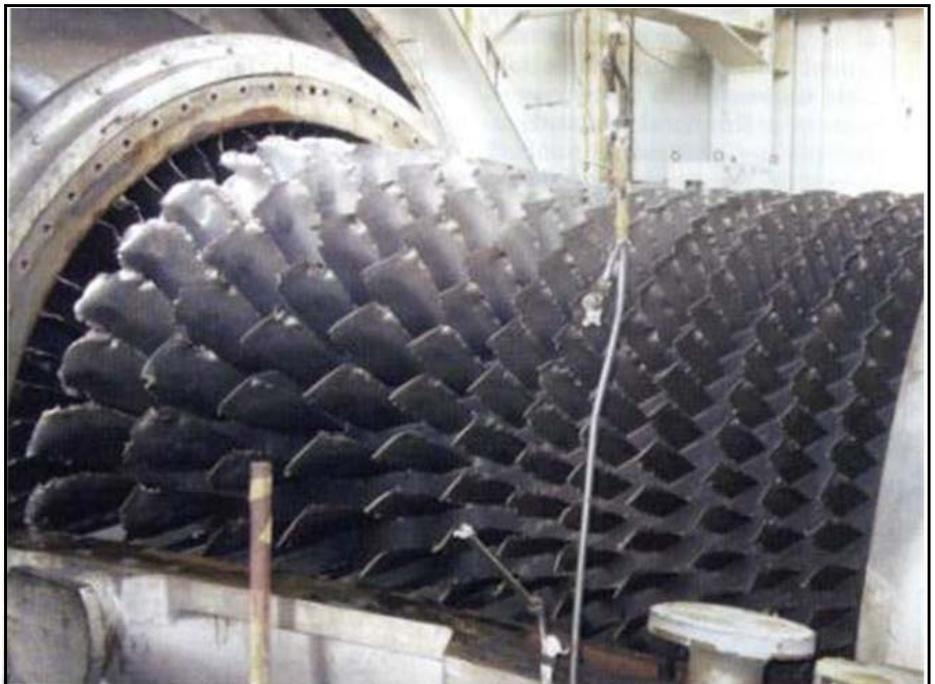
**Figure 1. Failure of a first-row blade showing the damage to every stage of the compressor.**
