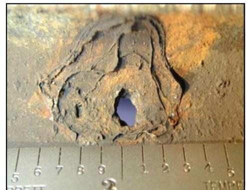
Figure 2. Typical Oxygen Pit.
