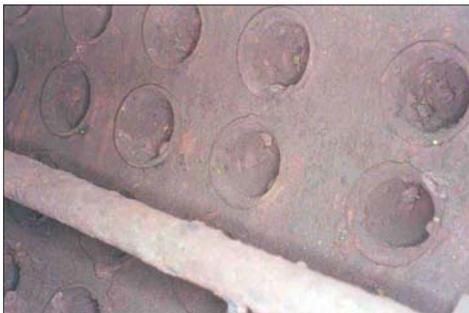
Figure No.1. Oxygen Pitting in Steam Drum.
