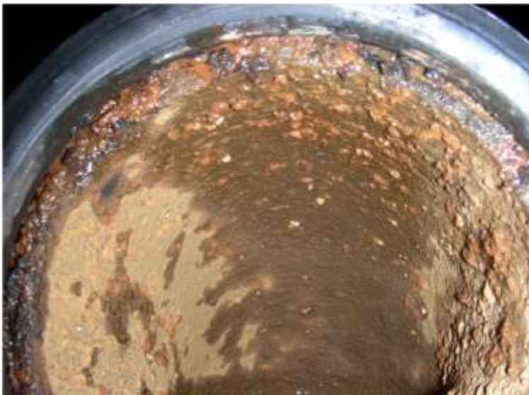
Figure 1. Photographs show examples of corrosion in galvanized piping hot, softened water service. (Continued on page 2)
