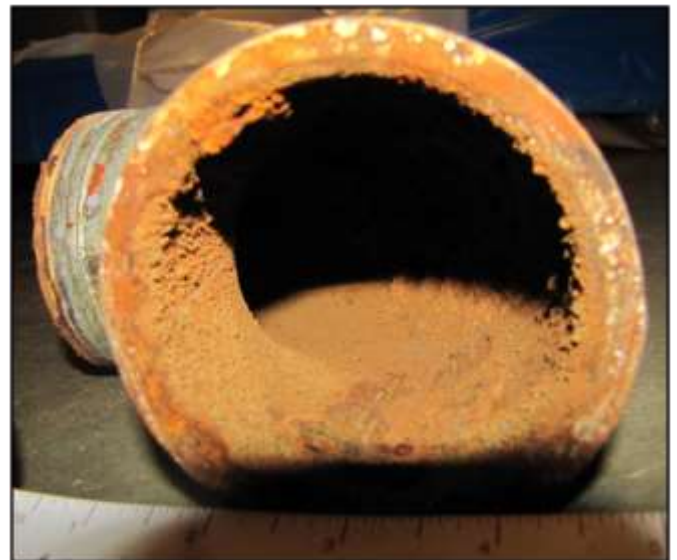
Figure 1. Photographs show examples of corrosion in galvanized piping hot, softened water service. (Continued on page 2)
